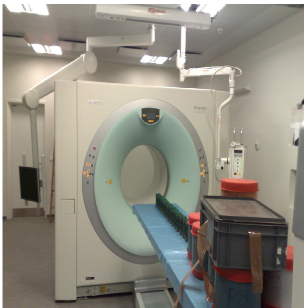
Fig.1. Detector+ X- ray source in rotation around the sample, it generates a 3 D image from a series of 2D images taken around a single axis of rotation as a non-destructive method
