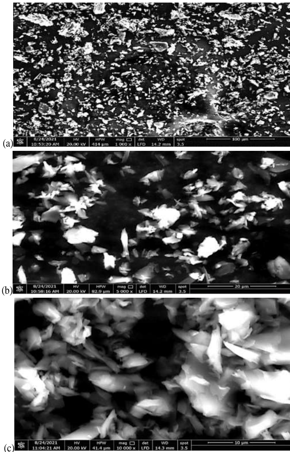
Fig. (7). Scanning Electron Microscope (SEM) images in of GO (a- 1000x, b- 5000x, c- 10000x).
