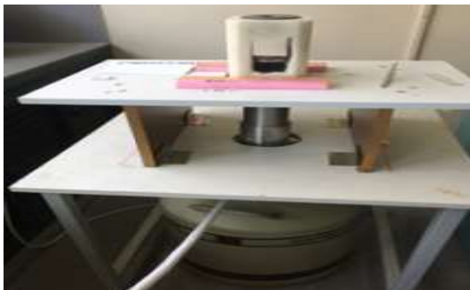
Fig. 2. The system used for gamma ray attenuation measurements.
