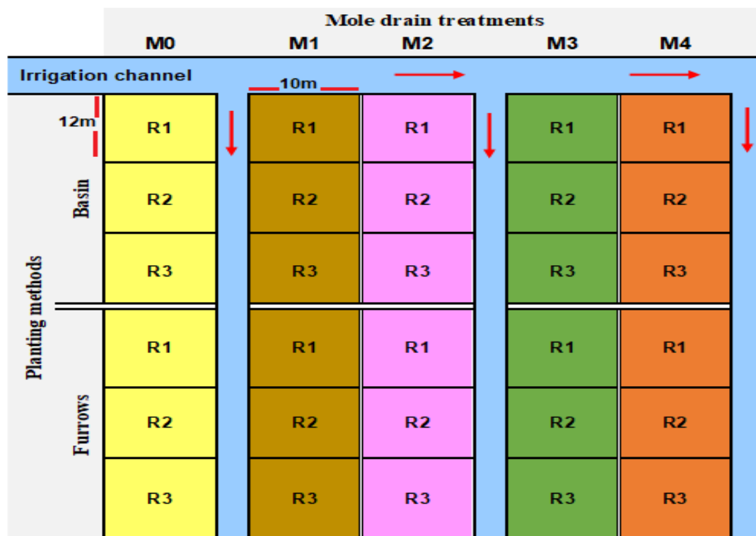
Fig. 1. Design of the studied treatments (M0=control without mole, M1=2m mole space with 30 cm depth, M2= 2m mole space with 40 cm depth, M3= 4m mole space with 30 cm depth, M4= 4m mole space with 40 cm depth, R= replicate).
